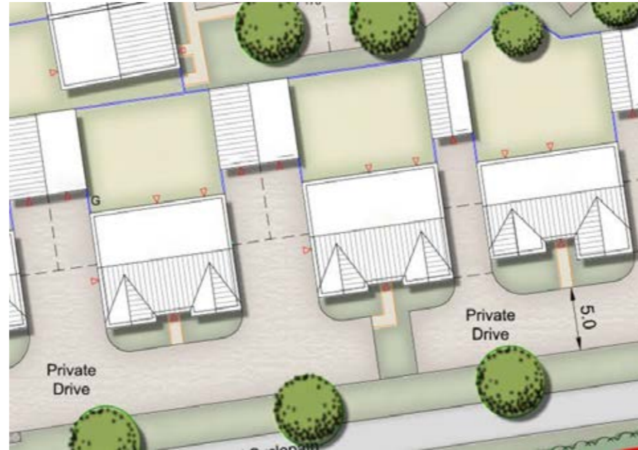
ON-PLOT GARAGE PARKING: ACCESS OFF A SHARED PRIVATE DRIVE ALLOWING FOR TANDEM AND 'TRIPLE' TANDEM PARKING; MIN. 6M IN FRONT OF THE GARAGE TO THE EDGE OF THE PRIVATE DRIVE
