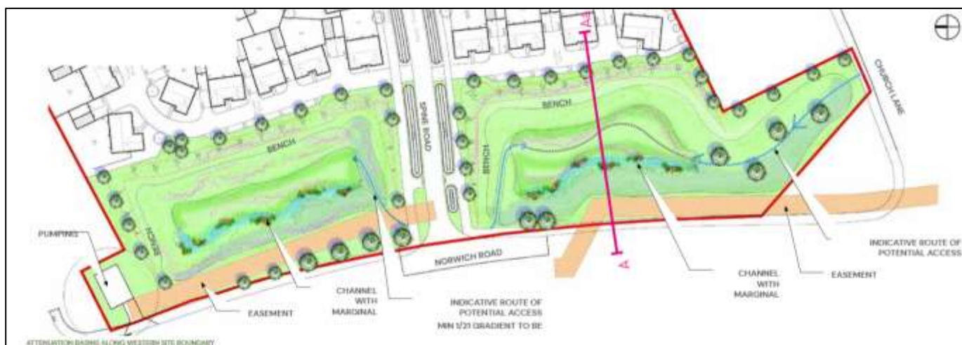
figure 17: An illustration from the Design Code showing how natural drainage basins are to be created that offer opportunities for enhanced biodiversity
