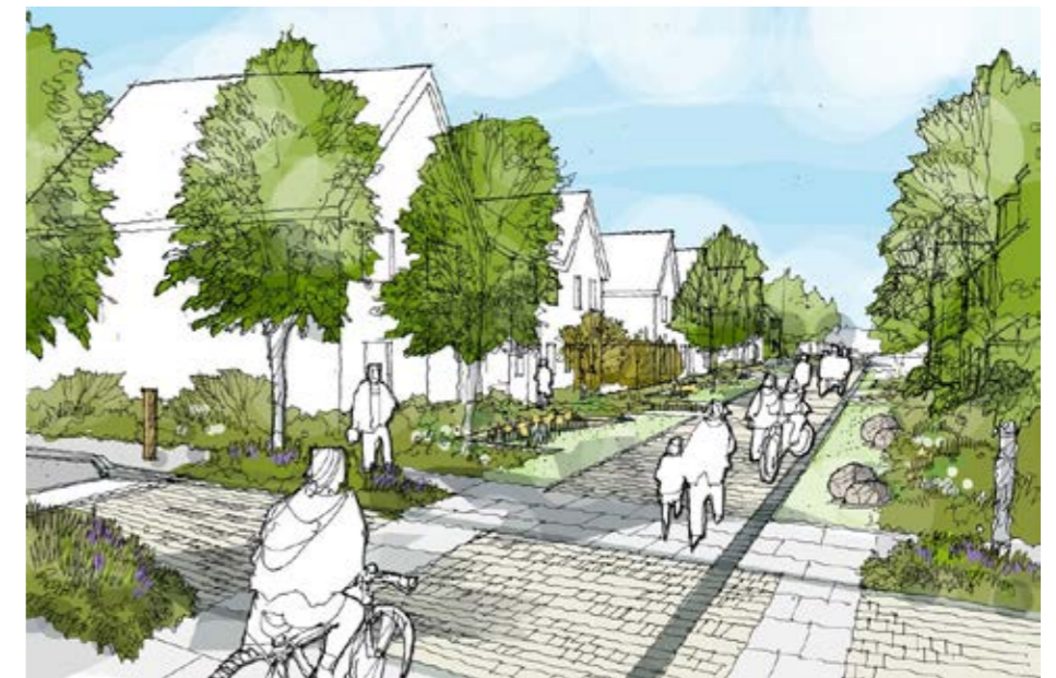
ILLUSTRATION OF A PEDESTRIAN/CYCLE PRIORITY CROSSING, INCORPORATING A PAVED RAISED TABLE AND SHRUB/TREE PLANTING TO ENCOURAGE A REDUCED VEHICULAR SPEED, ALLOWING A CONTINUOUS GREEN LINK THROUGH THE SCHEME.
